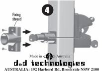
7. Take the Fixing Shroud and slide it over the Push-Button Lock (see left). Again, ensure push-rod is kept level. Drill 'pilot' holes and fasten the Fixina Shroud to the post using the two 19mmx10a (3/4"x10a) countersunk screws supplied USA: 7731 Woodwind Dr, Huntington Beach, CA 92647
